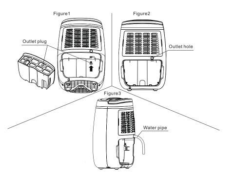
Note: Smoothly stretch the drainage, for if it is flat or twists together, drainage will not go on right; even the unit can not work normal. During the operation drainage pipe should never be in higher position than the hose connector.
